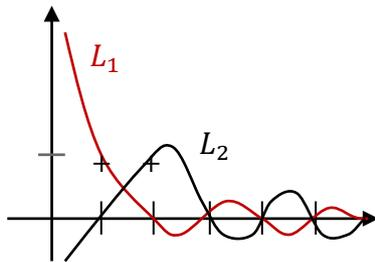
$$\left\{ \begin{array}{l} L_1(x) = \frac{(x-x_2)\dots(x-x_n)}{(x_1-x_2)\dots(x_1-x_n)} = \prod_{i=2}^n \frac{(x-x_i)}{(x_1-x_i)} \\ L_2(x) = \prod_{i=1|i \neq 2}^n \frac{(x-x_i)}{(x_2-x_i)} \\ \dots \\ L_n(x) = \prod_{i=1}^{n-1} \frac{(x-x_i)}{(x_n-x_i)} \end{array} \right.$$
